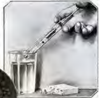
For office use, a handy syringe forces air through capsules of radium salts and into a glass of water, imparting radioactivity. Its sponsors claim, to the drinking water.
