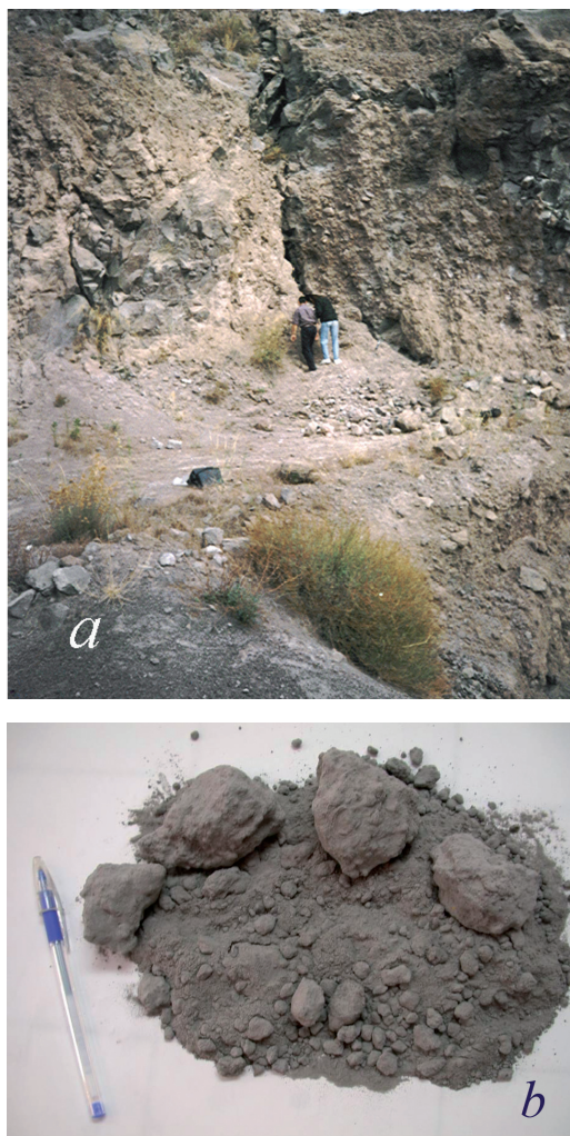
Fig. 1 – a) Extractive front of the “Il Calvario” quarry, where the vertical fractures present superficial mineralization of prismatic yellow fluoro-edenite amphibole; b) fine grained volcanic material of the “autoclastic breccia” (fractured and crumbled benmoreite lava) containing the fluorine fibrous amphiboles.
