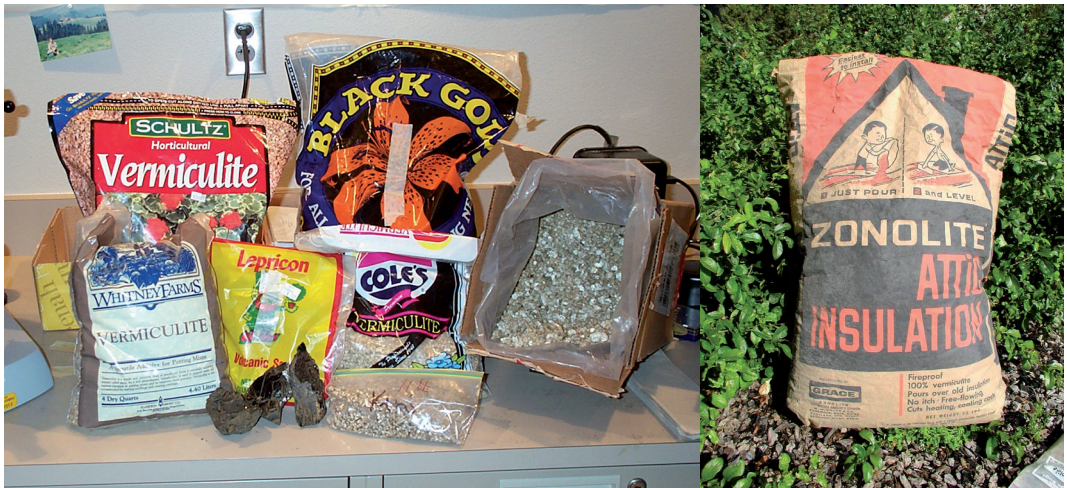
Fig. 2 – Photographs of the commercial vermiculite products used in this study (except for Thermorock). (left) These samples were purchased in local stores in the Moscow, Idaho USA area, and (right) a bag of unopened Zonolite obtained from the attic of building on the University of Idaho campus in Moscow, Idaho USA.
