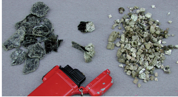
Fig. 1 – A photograph showing vermiculite (left) and expanded vermiculite (right). In the middle of the photograph a flake of vermiculite is shown, expanded on its right side, by applying heat from the lighter.
