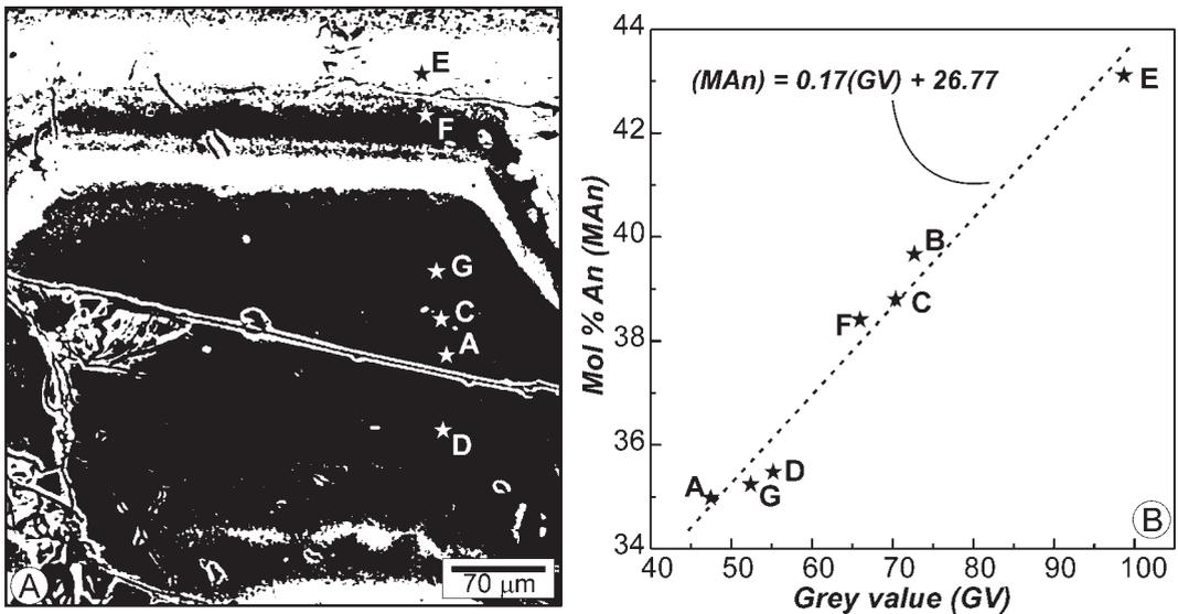
Fig. 2 – A) Example of back-scattered electron micrograph of a plagioclase crystal analyzed by electron microprobe (analyzed points indicated by white stars); B) linear correlation between grey intensity of analyzed points and mol.% An content. In the graph the equation of the linear fitting is also reported.
