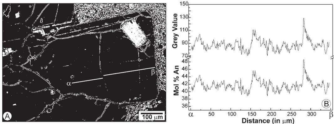
Fig. 3 – A) back-scattered electron micrograph of a plagioclase crystal from which the concentration profile is extracted (white line); B) concentration series along the transect  $\alpha$ – $\beta$  in A. In the graph are reported both the grey intensity and the mol. % An variation.
