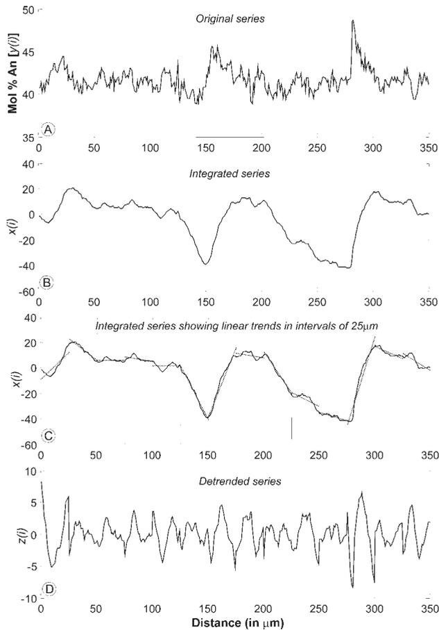
Fig. 5 – Main steps of the Detrended Fluctuation Analysis used to quantify the oscillatory zoning in plagioclase crystals applied to the compositional time series shown in Figure 3B. See text for details.
