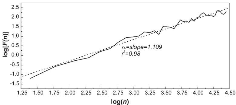
Fig. 6 – Graph showing the variation of  $\log[F(n)]$  versus  $\log(n)$  for the time series reported in Figure 5A. Scaling exponent  $\alpha$  is calculated as the slope of linear fitting of data.
