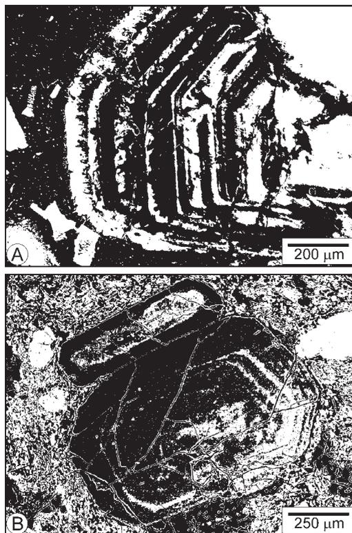
Fig. 1 – Examples of oscillatory zoning in plagioclase crystals from the studied lava flows: A) cross polarized optical micrographs of a crystal from the CPS lava flow; B) back-scattered electron micrograph of a crystal from the SR lava flow.
