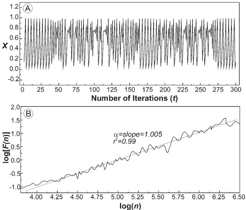
Fig. 9 – A) Time series of  $X$  values obtained by using the logistic map with  $r=3.9601$ ; B) Graph showing the variation of  $\log[F(n)]$  versus  $\log(n)$  for the time series in A. Scaling exponent is calculated as the slope of linear fitting of data in the scaling region from ca. 4.0 to ca. 6.5.
