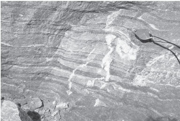
Fig. 5 – Aymaville Marble outcrop at Pessa Alta quarry. Calcite (light) and dolomite (dark) levels, of different grey tonality are distinguishable.
