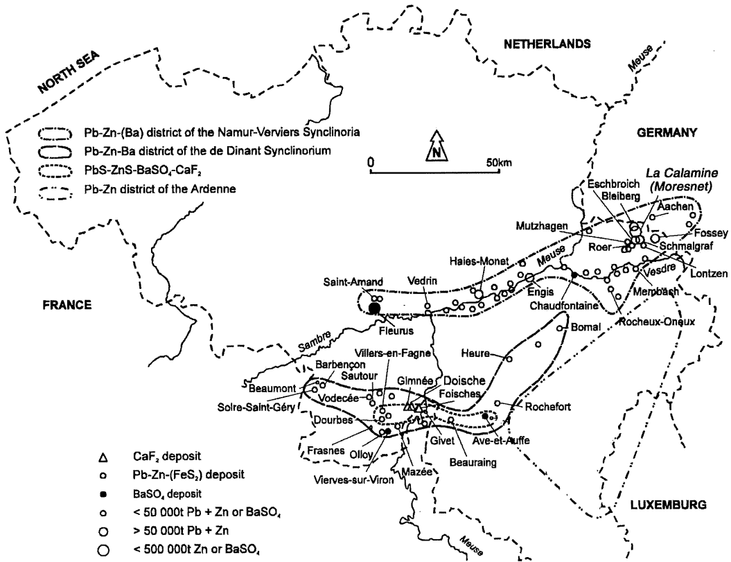
Fig. 1 – Sketch map of the Zn-Pb districts in Belgium, showing the location of the primary and secondary deposits (modified from Dejonghe, 1998).
