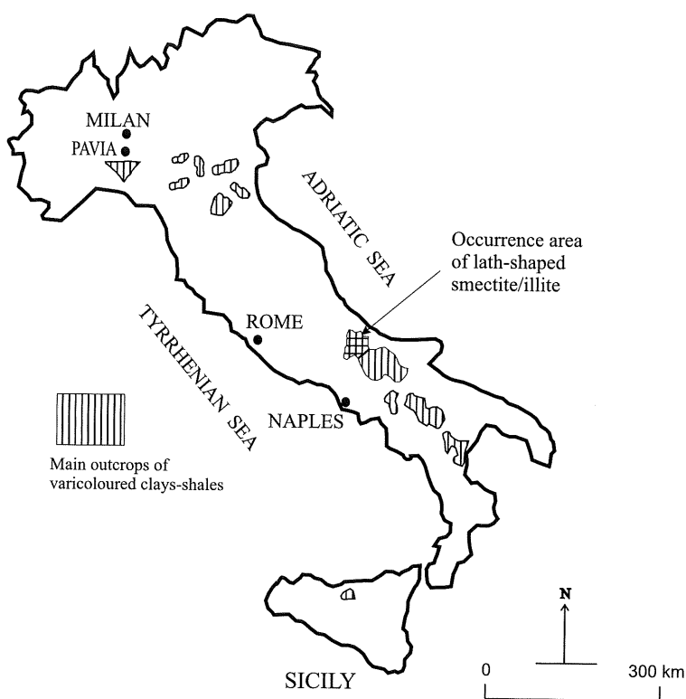
Fig. 1 – Occurrences of varicoloured clays-shales along the Italian Apennines strip.
