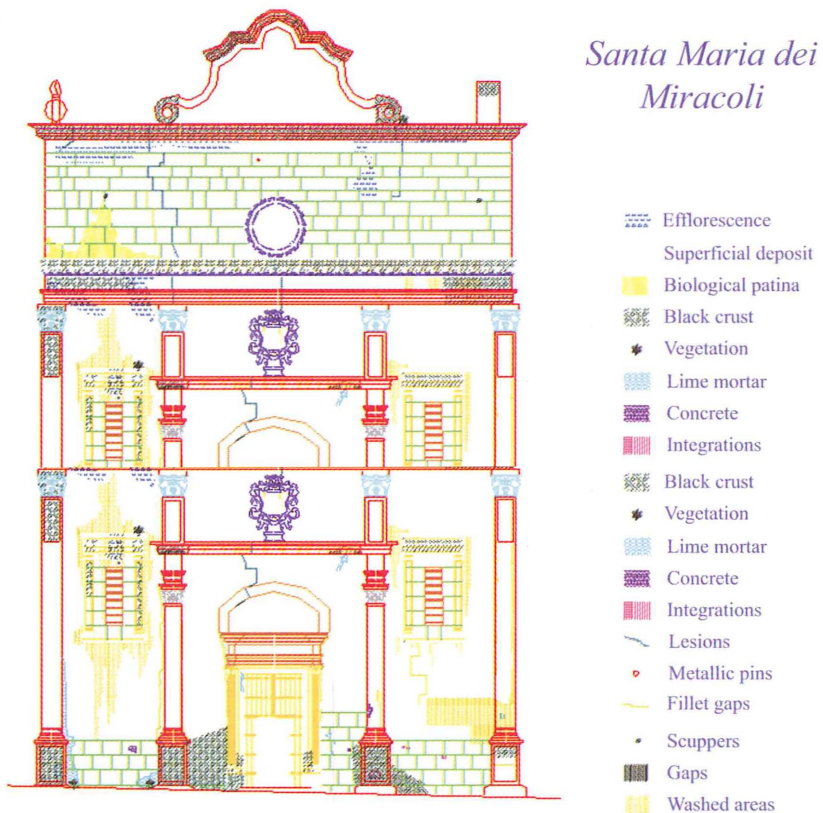
Fig. 4 – Graphic restitution of the photogrammetric relief of the church of Santa Maria dei Miracoli showing the state of defects.
