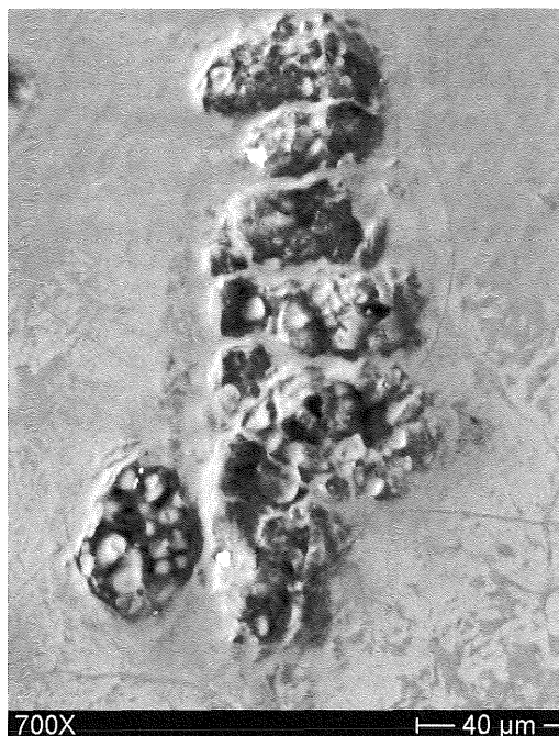
Fig. 8 – Silicon- and aluminium-rich inclusions inside mineralized iron rod.
