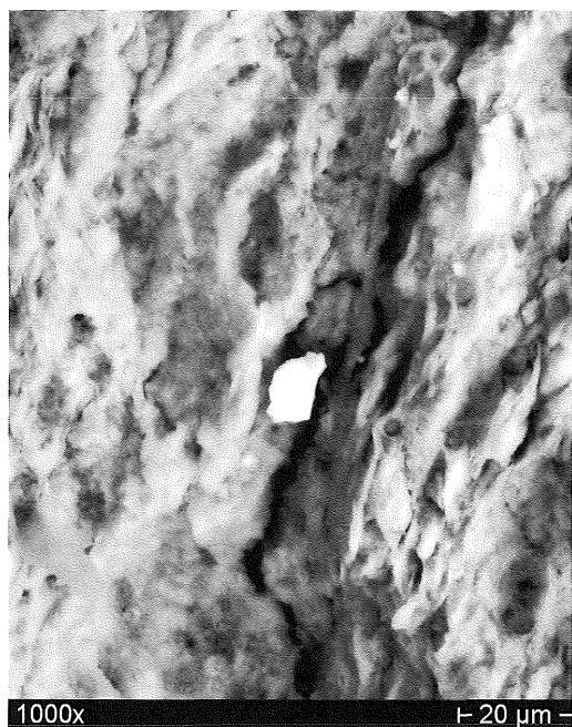
Fig. 12 - Photo of the grey bucchero's mixture backscattered electrons); there is a greater abundance of iron compared to the compositions of the mixtures of the architectural decoration and sculpture in terracotta production. This is evident from the distribution of this element in the map.
