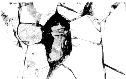
Figs. 5-6 – 5) Narrow vein around a primary orthopyroxene with primary inclusion-spinels (poikilitic texture, Szt-1034). The vein is composed of fragments of primary orthopyroxene, secondary clinopyroxene, glass and vugs. II N. M=20x. 6) Texturally equilibrated amphibole grain in Szt-1106 showing signs of decomposition involving the formation of secondary clinopyroxene and glass. II N. M=40x.
