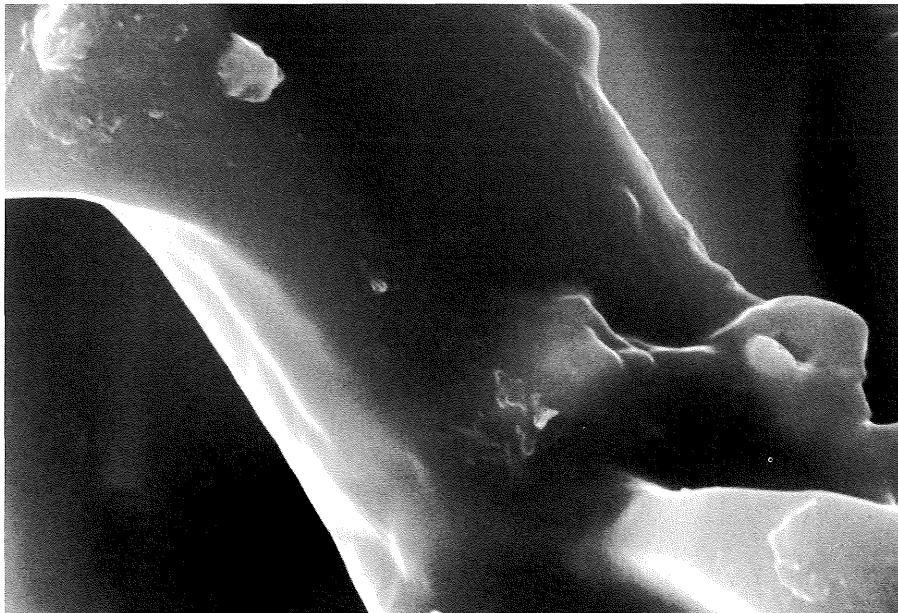
Fig. 4 – SEM magnified images of PARIS1 after the interaction with the epoxy resin at a different magnification showing a clear change in the microstructure of the material.
